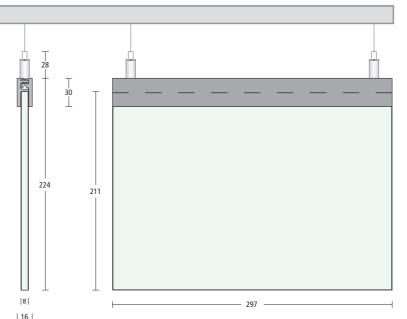
Ceiling suspended signposts in the system **transparenz** offer the special attraction of a valuable information transmission. Even if they appear light due to the transparent surface, the load-bearing capacity of a suspended ceiling with the weight of the panes must be taken into account. Ceiling signs that are seen from both sides require a back cover to avoid mirror writing.
